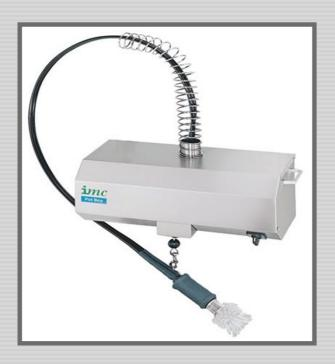
Pot Boy uses a powered nylon brush head to remove stubborn deposits from pots and pans. Mounted over a sink, it is always ready for use. Lightweight and easy to use, the operator simply guides the brush around the item being cleaned. Safety is assured as the brush head is driven by a hydraulic circuit providing both electrical isolation and overload protection
